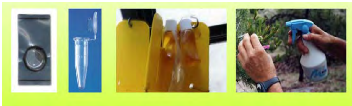
Fig. 1 Release devices used (left to right): Polyethylene bubblecaps ( Pityol,Hexenol ), Eppendorf tubes ( Conophthorus ), Polyethylene vials (4-AA) and Sprayable wáter suspensi3n (microcapsulate Verbenone ).
