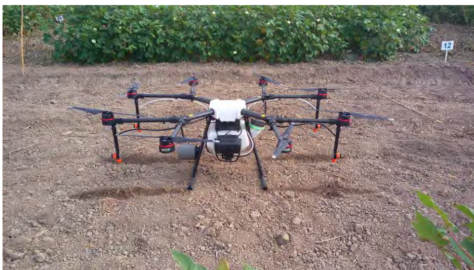
Fig. 1 UAVs sprayer, DJI Agras MG-1 used Global Navigation Satellite System and Real-Time Kinematic (GNSS RTK) navigation technology.
