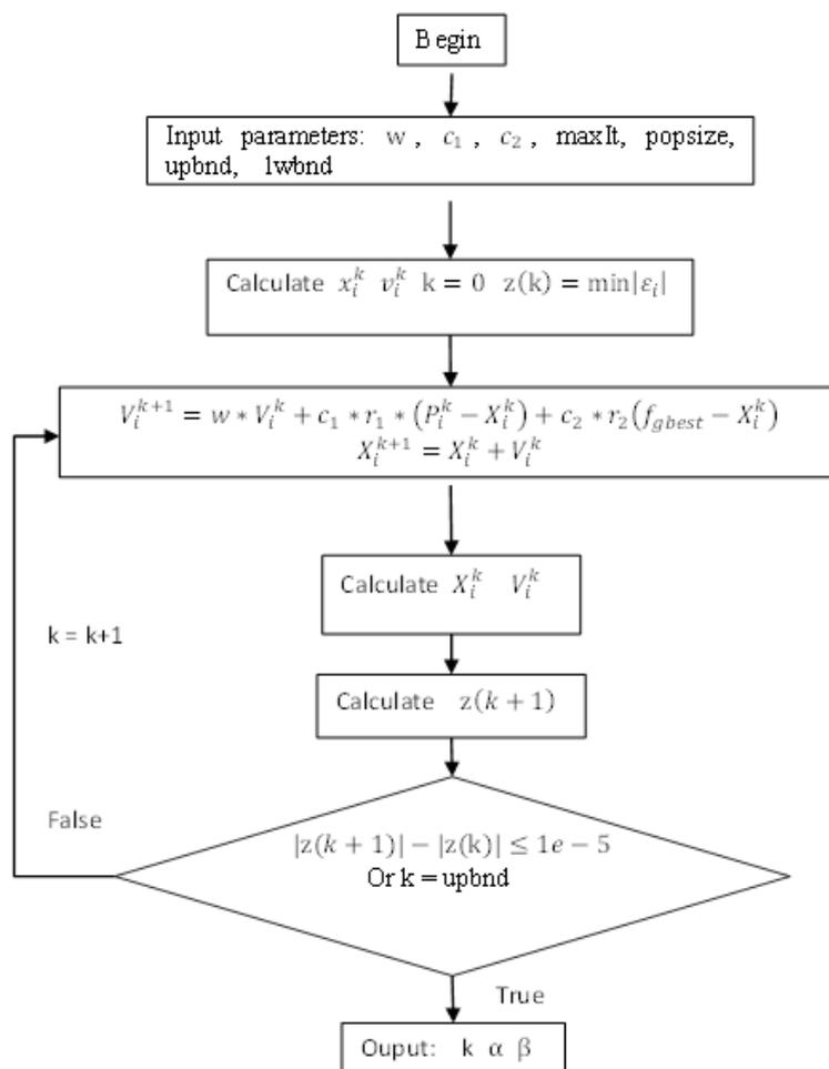
Fig. 1 Computation flowchart of Particle Swarm Algorithm in this paper.
