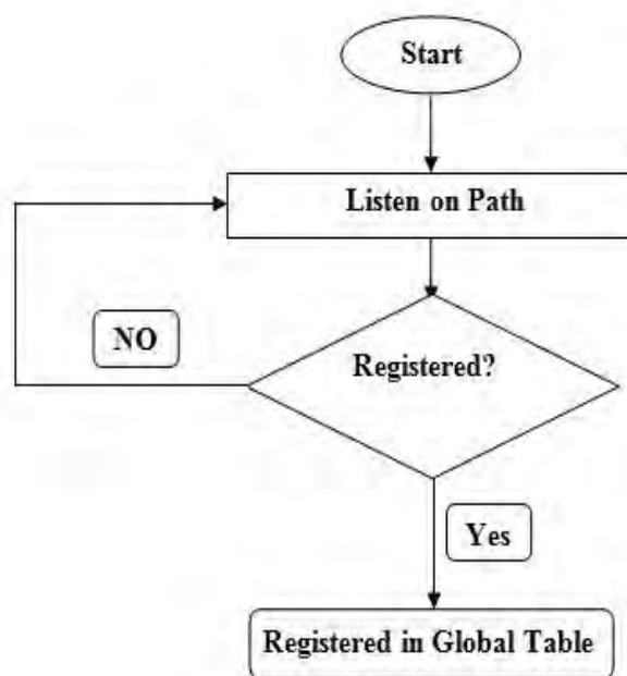
Fig. 6 Listener algorithm flowchart in distributed frame workload.
