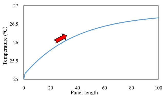
**Fig. 5** Experimental result of the airflow temperature gradient along the length of the thermal collector.
