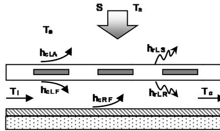
Fig. 3 Heat transfer coefficient of different parts of the of Single path bifacial PVT collector (Ooshaksaraei et al., 2017).
