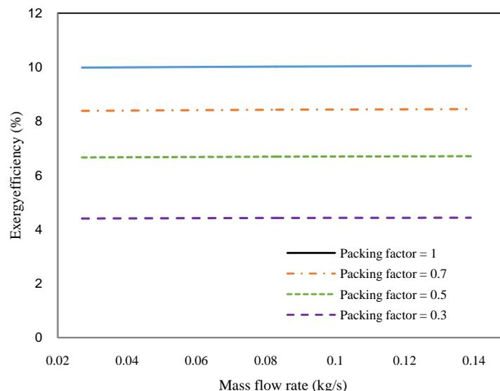
**Fig. 7** The total exergy efficiency of bifacial PVT collector.
