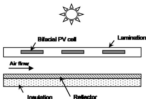
**Fig. 2** Cross section schematic of the single path bifacial PVT collector (Ooshaksaraei et al., 2017).
