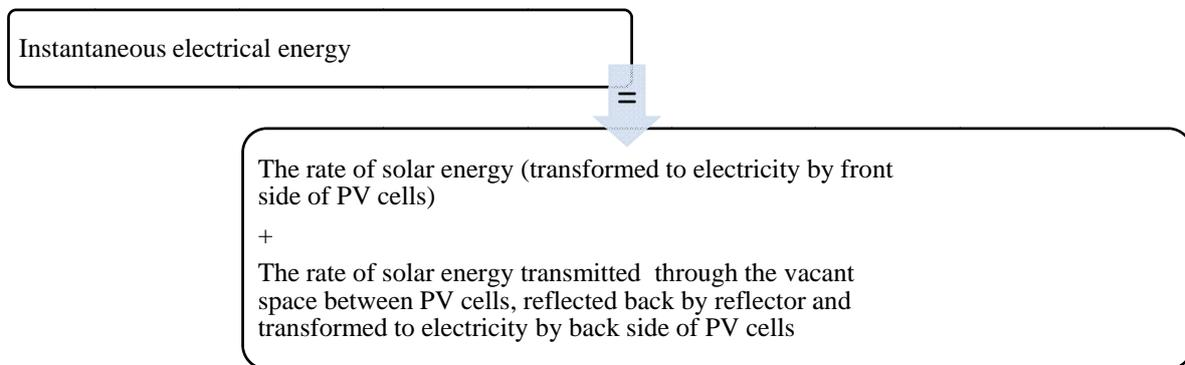
where “P” proposed that solar cells covers only a portion of the PV panel but not the entire surface of it. The overall electrical efficiency of the PV panel depends on the packing factor (P) in which when it increases the temperature of the PV panel will reduce (Chow, 2003; Zondag et al., 2003; Agrawal and Tiwari, 2011). In addition, the thermal exergy of a solar collector can be calculated through equation 11 (Borel and Favrat, 2010)
