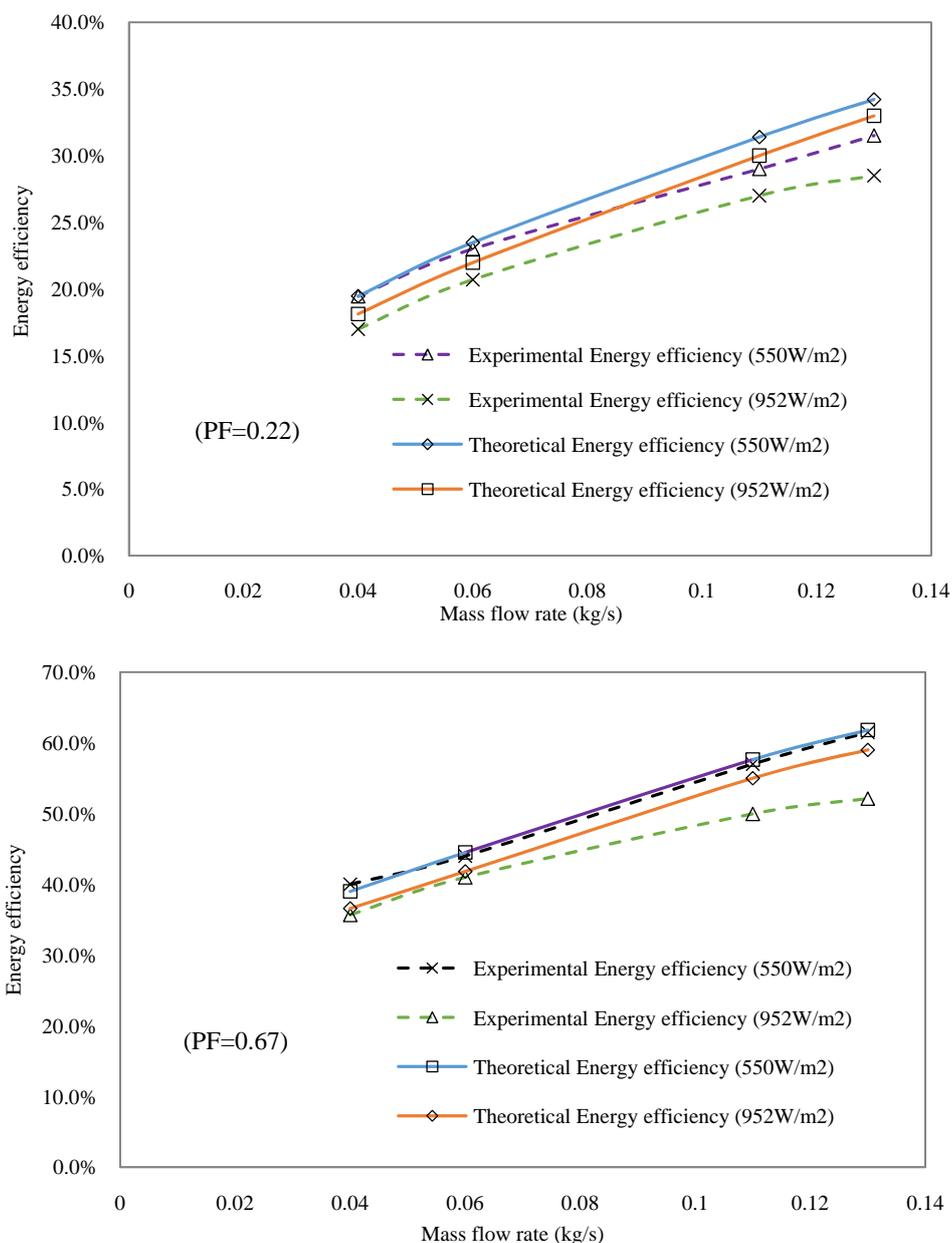
**Fig. 6** Theoretical and experimental photovoltaic thermal efficiency comparison for packing factors 0.22 and 0.67.
