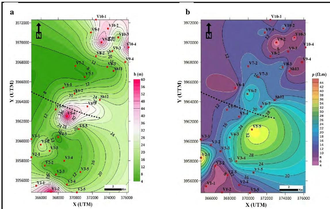
**Fig. 7a:** Thickness of Quaternary aquifer ( $h$ ) in thirty four VES points in the research area, **b:** Resistivity ( $\rho$ ) of the Quaternary aquifer in thirty four VES points in the research area.
