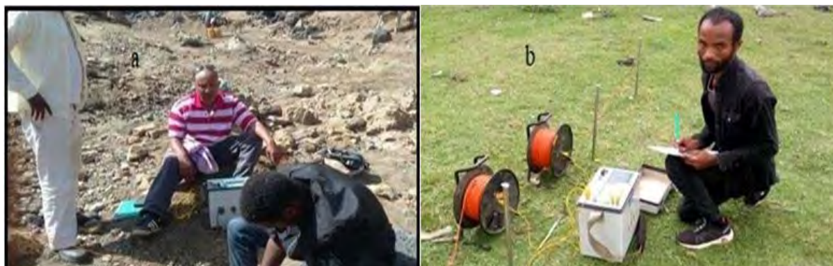
Fig. 5 Photographic view of vertical electrical sounding (a) and electrical imaging tomography (b).
