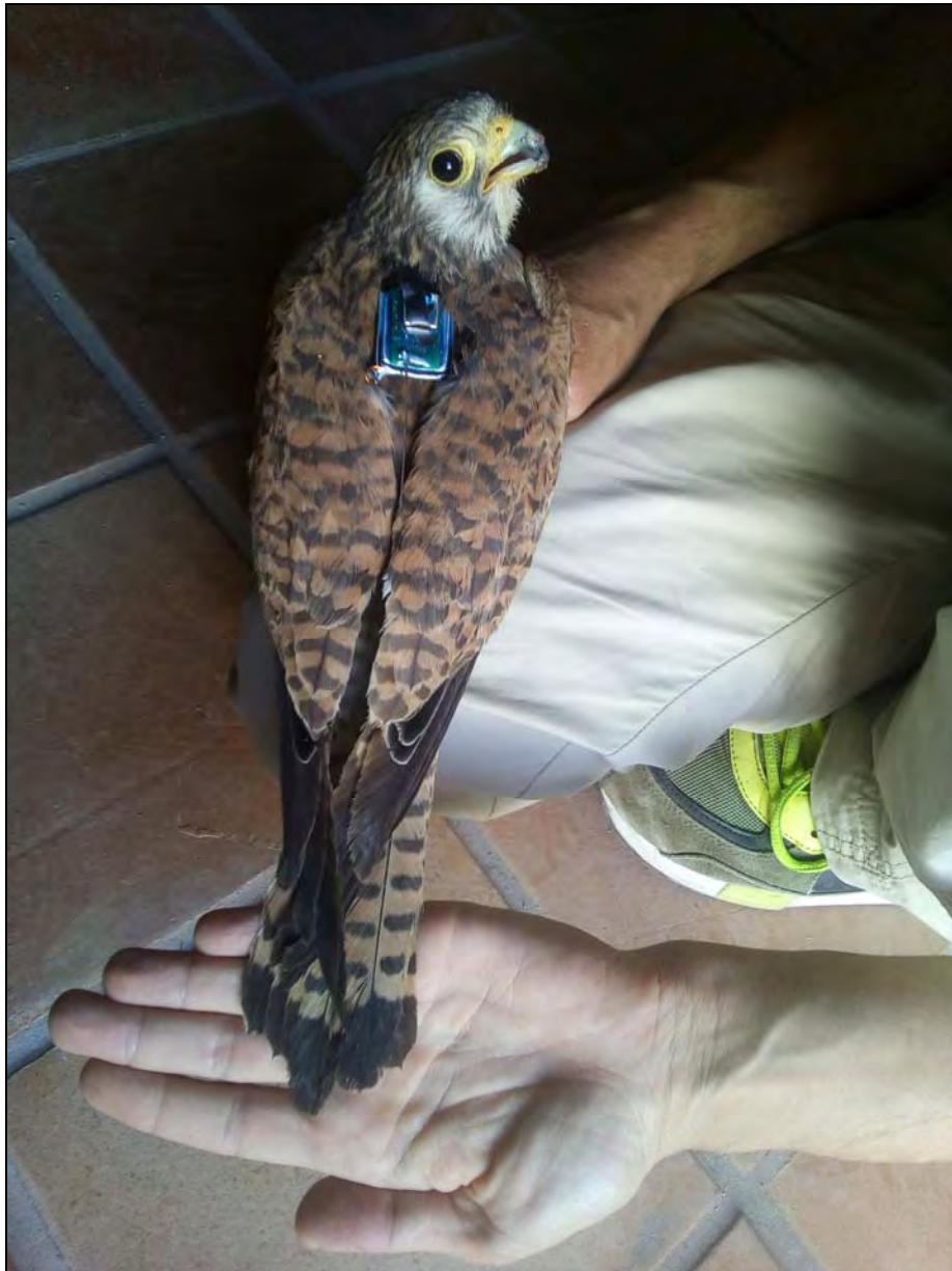
Fig. 2 We used TechnoSmart GiPSy-4 data-loggers (23×15×6 mm, 5 g weight) that provided information about date, time, latitude, longitude, altitude and instantaneous speed.
