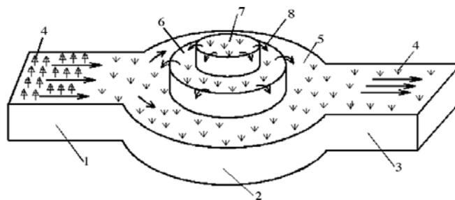
**Fig. 2** Schematic layout of Towery hybrid constructed wetland: 1, first stage; 2, second towery stage; 3, third stage (discharge); 4, wetland plants; 5, bottom circular cell; 6, middle circular cell; 7, upper circular cell; 8, cascade (Fenxia and Li, 2009).
