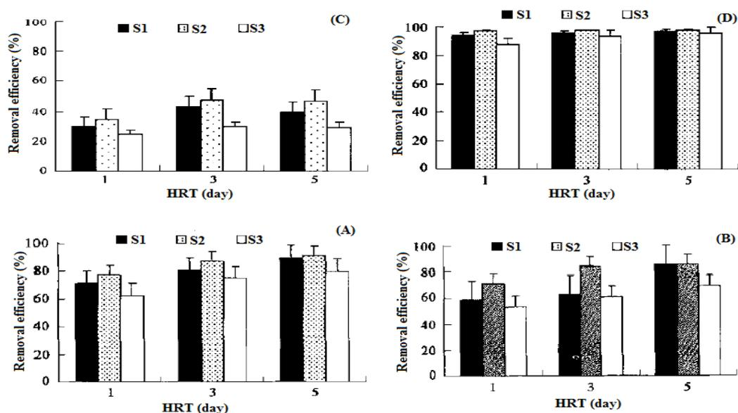
**Fig. 3** Mean removal efficiency of COD (A), BOD<sub>5</sub> (B), TN (C) and TP (D) at different HRT in hybrid CW systems (S1, S2, S3) (Cui et al., 2006)
