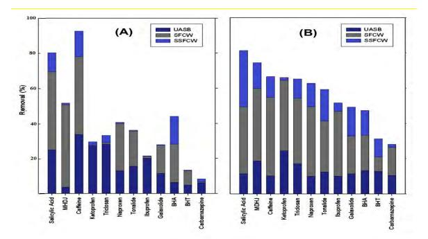
**Fig. 4** Relative mass removal of dissolved PPCPs according with treatment stage, UASB, FWS, HSSF (A) winter (February 2008) (B) summer (June–July2009). Compound identification as following; MHDJ: methyl dihydrojasmonate, BHA: butylated hydroxylanisole, and BHT: butylated hydroxytoluene (Contreras et al., 2011)
