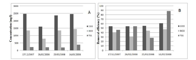
**Fig. 6** average pollutants influent concentration (A) and average removal efficiency (B) at different period of system operation (Comino et al., 2011)
