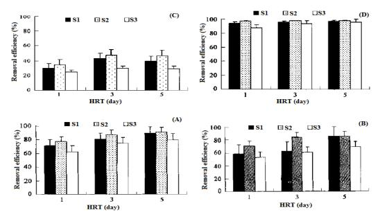
**Fig. 3** Mean removal efficiency of COD (A), BOD<sub>5</sub> (B), TN (C) and TP (D) at different HRT in hybrid CW systems (S1, S2, S3) (Cui et al., 2006)
