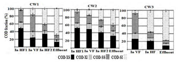
Fig. 5 COD fraction in different sampling point of three hybrid CWs (1, 2, 3) (Tuszynska et al., 2008).
