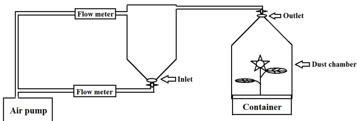
Fig. 1 Schematic presentation of the dust generator and dust chamber has used in present study.
