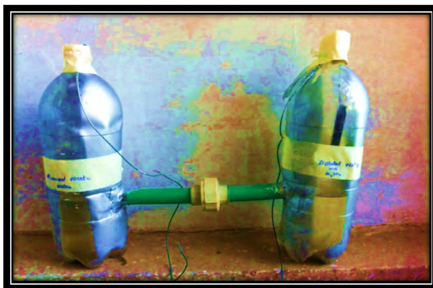
Fig. 3 Shows MFC system constructed for production of electricity.
